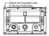
Connect the required cables to the rear of the Display Unit. If there is no NMEA2000 connections in your configuration, fit the supplied NMEA2000 connector cap to the NMEA2000 connector, at the rear of the Display Unit.
