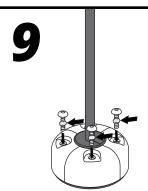
Apply marine sealant to the four allen head screws and tighten.
