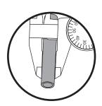
Measure your cable diameter and select the appropriate drill tube provided. Cable diameter +.01/-.03
