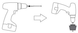
Insert drill tube into drill motor, and leave enough length to get through the tapered plug.
