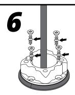
Secure the base to the mounting surface with the four screws.
