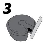
Wrap the rubber grommet around the electronic cable.
