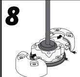
Combine the two halves of the outer shell. These will snap together with a click. Be sure to stagger the seams as shown by the two black arrows.
